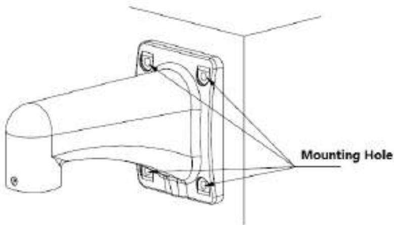
**Step 3** Install the speed dome on the wall-mounted bracket. See Figure 3-5. For details about speed dome installation, see "2.6 Speed Dome Installation".
