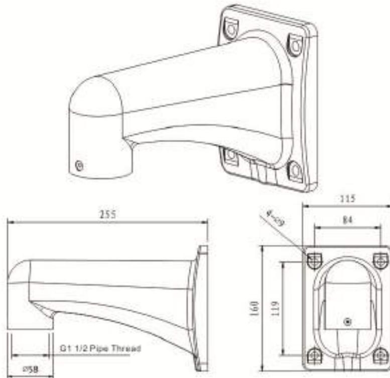
Figure 3-3 Dimension of quick mounting connector (mm)
