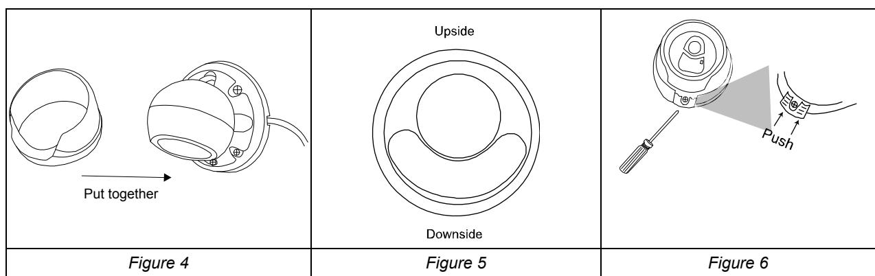
Step 5: Rotate the case to the base and make sure it's fastened. (Refer to *Figure 6*)
