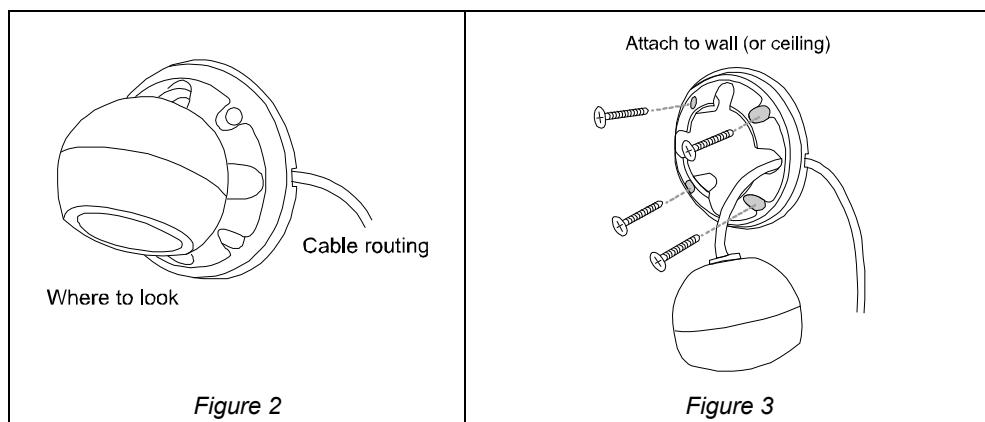
Step4: Put together the case and the lens, and slightly adjust the camera lens. Make sure it faces your target surveillance area.
