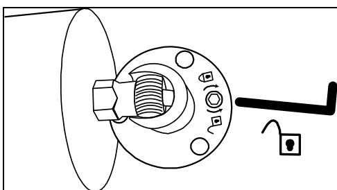
Step2: Locate where to install this camera, and fasten the bracket to the ceiling or wall. Then, adjust the viewing angle of the camera, and fasten the screw to secure the joint lock of the bracket.
