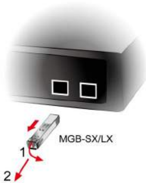
Figure 2-8 How to Pull Out the SFP Transceiver
