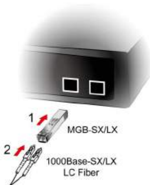
Figure 2-7 Plug in the SFP transceiver
