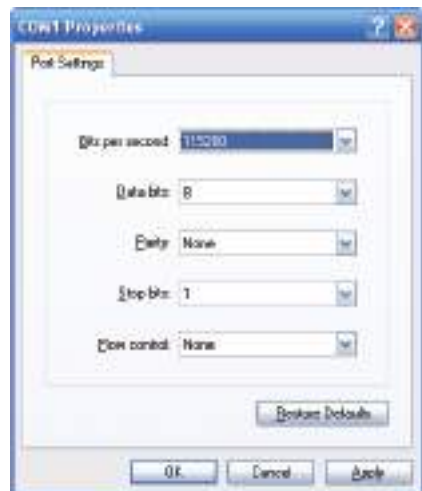
Figure 4-2: COM Port Configuration
