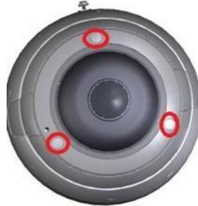
**Figure 6.** Site of screws on camera front cover
