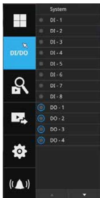
Click on the DI/DO button to display the full list of all DI and DO signals (whether they are connected or not) from all cameras in the configuration. If a digital input signal is triggered, e.g., the DI-4 on the left, its indicator will turn solid white.
