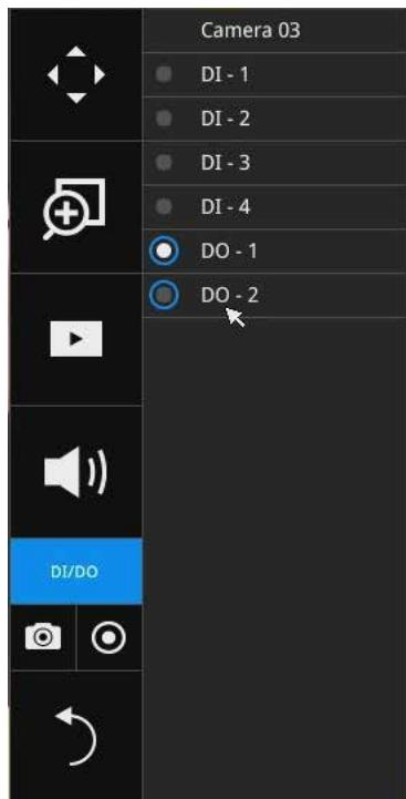
The DI/DO panel provides a glimpse of all DI and DO signal statuses from the connected cameras. You can manually trigger a digital output by clicking on its indicators.
