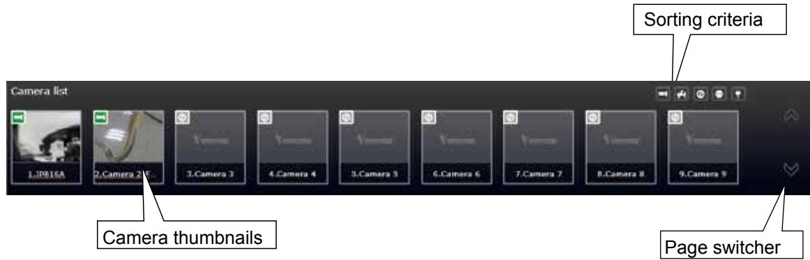
Depending on the size and screen resolution of your monitor, the snapshots of 8 cameras are displayed in this panel. If a user logged in using a credential of a limited access, he may only see cameras that he can access instead of all of the cameras.
