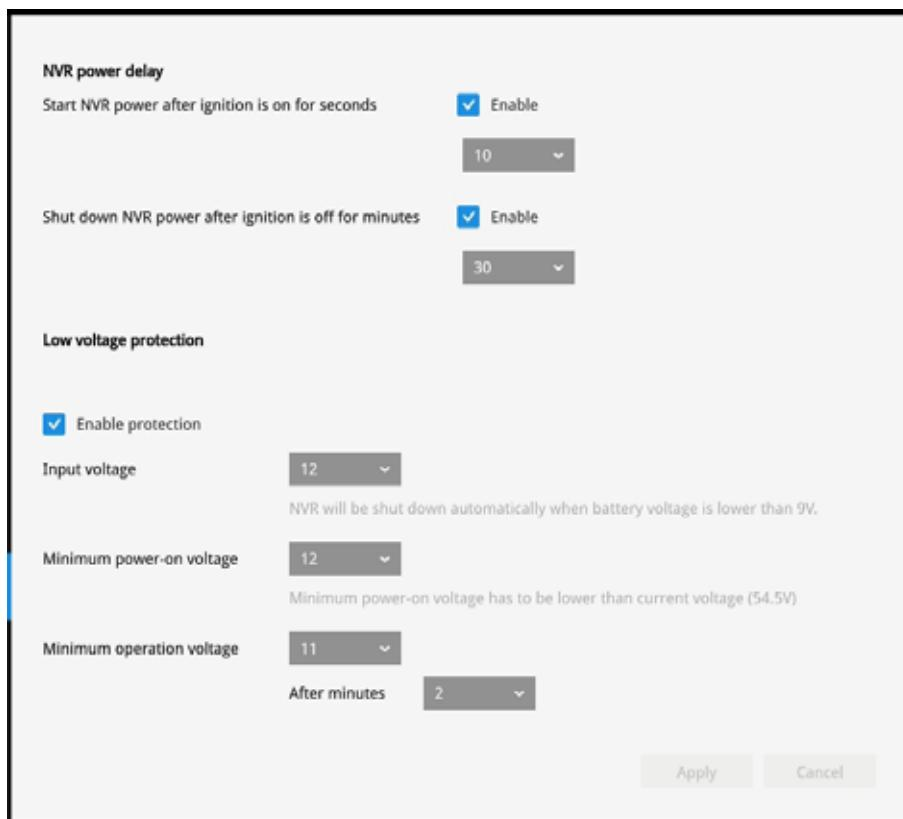
The low voltage protection feature enables the system to be powered down after the low voltage condition persists for a configurable period of time.
