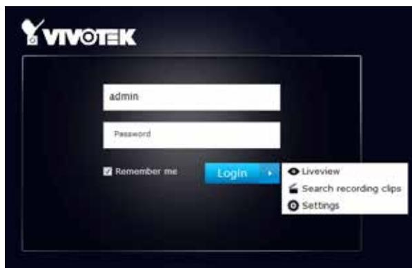
The NVR system features a simple UI structure which consists of a Liveview window, a Playback utility, and a system Settings window. Once logged in, you can move from one window to another by selecting the hot link buttons on the upper right of the screen.
