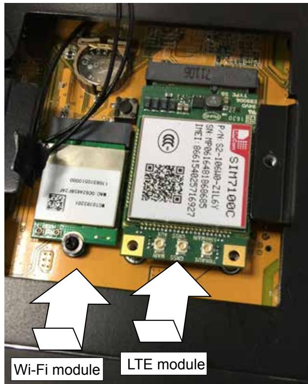
Secure the installation by driving 3 screws.
