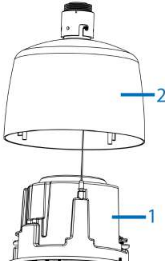
Figure 22 Camera housing and pendant mount
