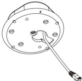
4. Pass cables through the waterproof rubber seal and complete all cabling requirements as documented in the camera QIG.
