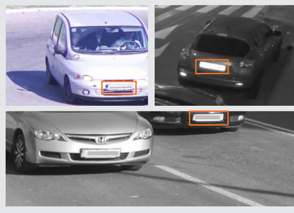
Too much light. Either adjust the iris or shutter speed. Night time: dim the IR or set AGC to Low.
