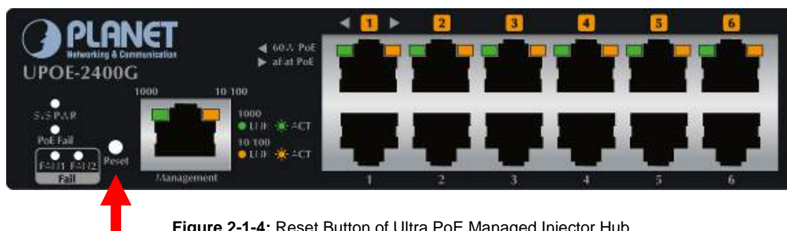
Figure 2-1-4: Reset Button of Ultra PoE Managed Injector Hub
