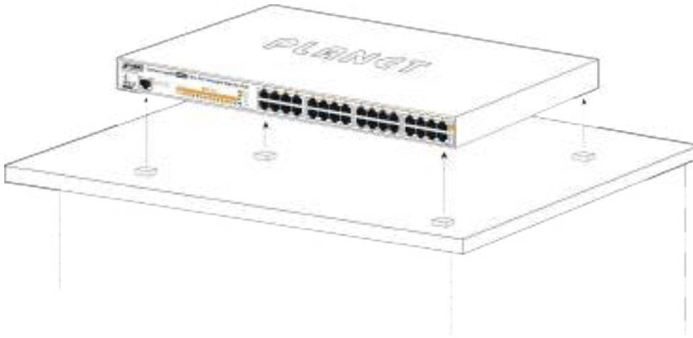
Figure 2-2-1: Desktop Installation of the Ultra PoE Managed Injector Hub
