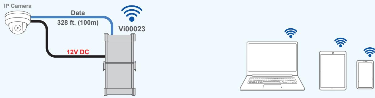
The Vi00023 enables connecting the non PoE cameras to any wireless device using a WiFi connection.
