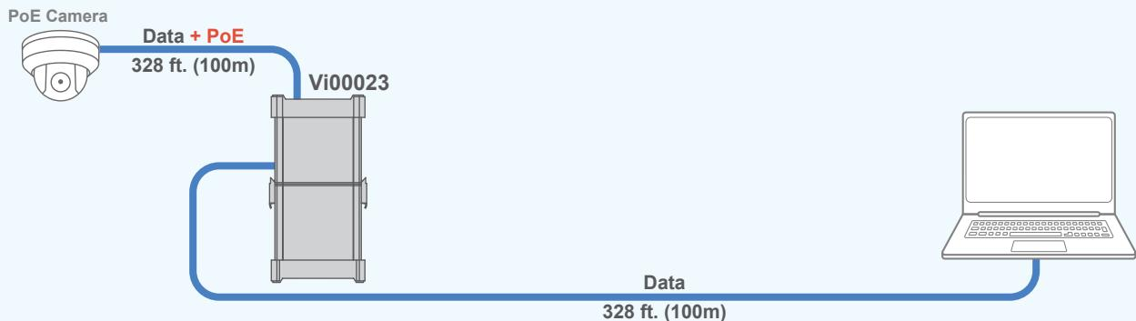
The Vi00023 enables connecting to a laptop using a wired connection.
