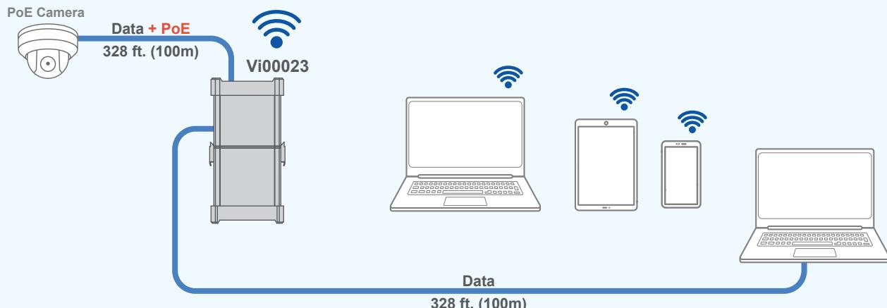
The Vi00023 has a built in switch that makes it possible to connect the IP camera to a network of wired and wireless devices.
