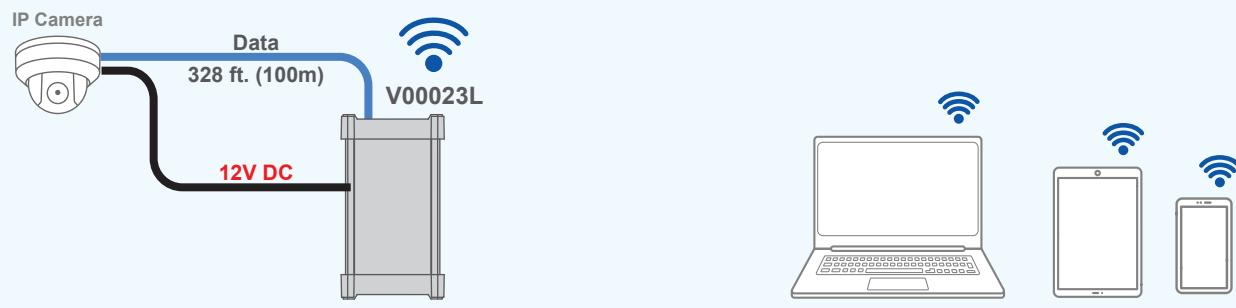
The Vi00023L enables connecting the non PoE cameras to any wireless device using a WiFi connection.
