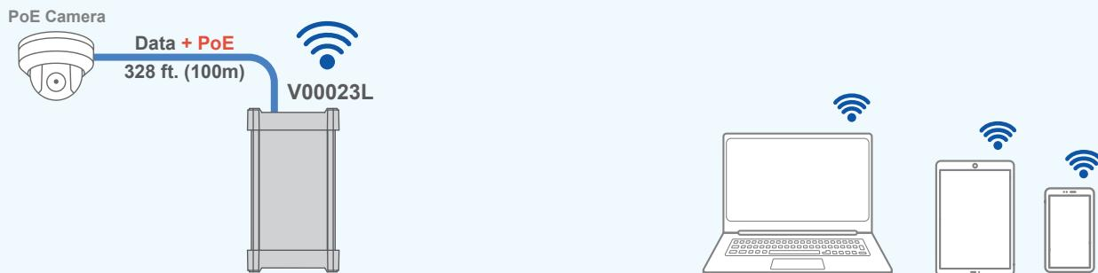
The Vi00023L enables connecting the PoE cameras to any wireless device using a WiFi connection.
