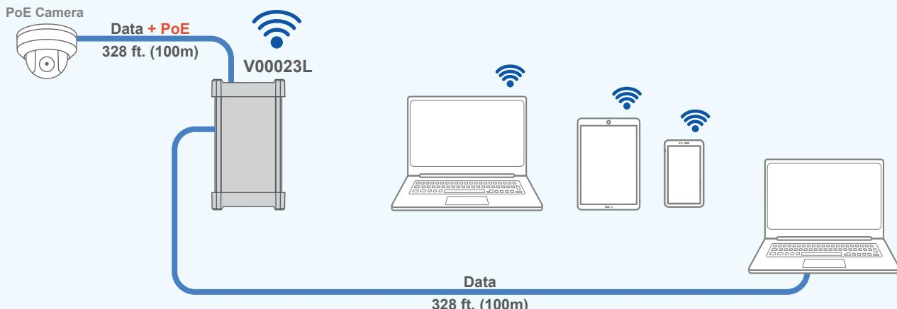
The Vi00023L has a built in switch that makes it possible to connect an IP camera to a network of wired and wireless devices.
