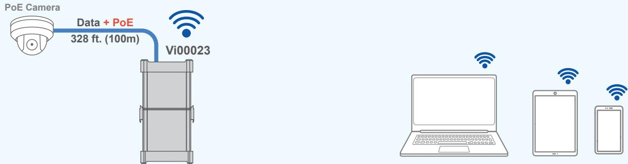
The Vi00023 enables connecting the PoE cameras to any wireless device using a WiFi connection.
