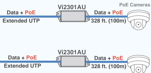
The NetMux™ Vi00103 along with Vi2300 series can connect two cameras at extended UTP distances.
