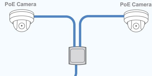
The NetMux™ Vi00103 can connect two cameras at standard UTP distances over a single cable.
