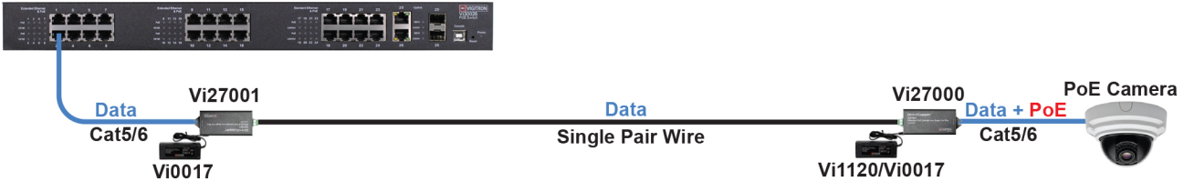
Both the Vi27001 and the Vi27000 can use local power supplies to power themselves and provide PoE to the IP camera .
