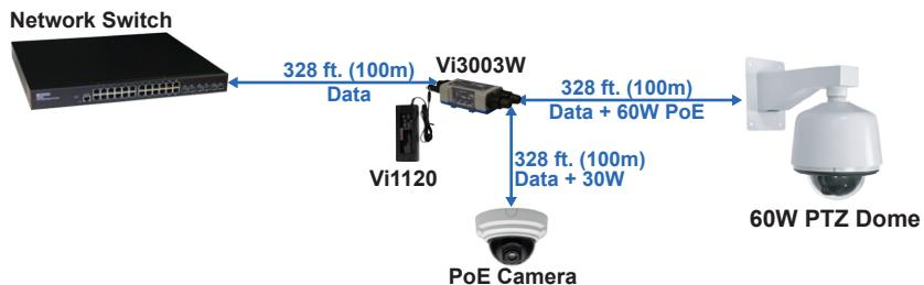
*Vi3003W allows for the transmission of two cameras over a single camera run or adding a new camera close to an existing camera.*
