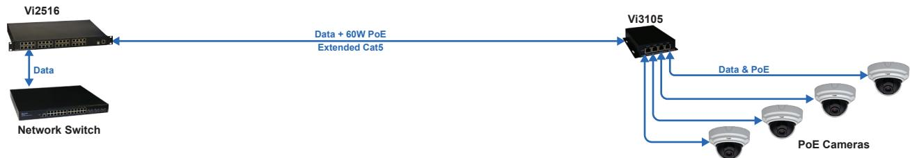
The Vi3105 can receive data and 60W PoE power over extended distance UTP up to 2,000 ft. at 100Mbps and power up to 4 cameras.
