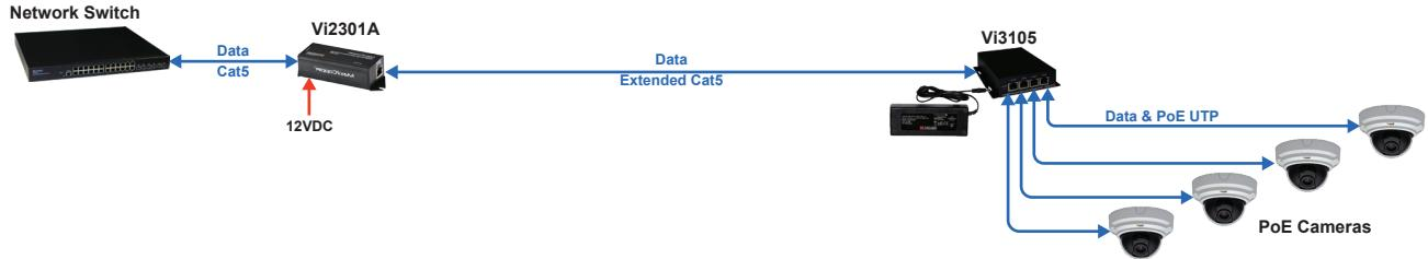
The Vi3105 can receive data over extended distance UTP up to 2,000 ft. at 100Mbps and power 4 PoE cameras using local power supplies.
