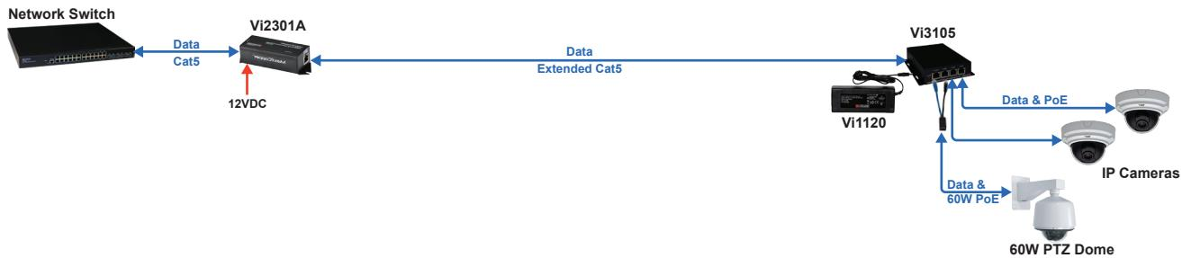
The Vi3105 can receive data over extended distance UTP up to 2,000 ft. at 100Mbps and power 60W PoE cameras using the Vi0015 combiner cable and a local power supply.
