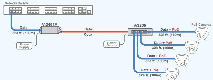
The Vi3205 can receive data over Coax up to 3,000 ft. at 100Mbps and power up to 4 cameras using a local power supply.
