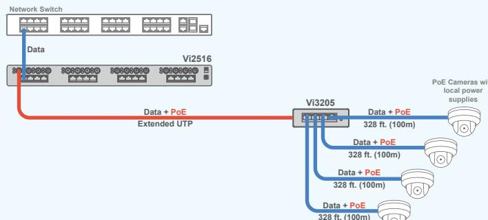
The Vi3205 can receive data and PoE power for powering itself over extended distance Coax up to 3,000 ft. at 100Mbps. The cameras use local power supplies.
