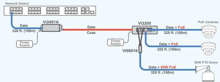
The Vi3205 can receive data over extended distance Coax up to 3,000 ft. at 100Mbps and power 60W PoE cameras using the Vi00016 combiner cable and a local power supply.
