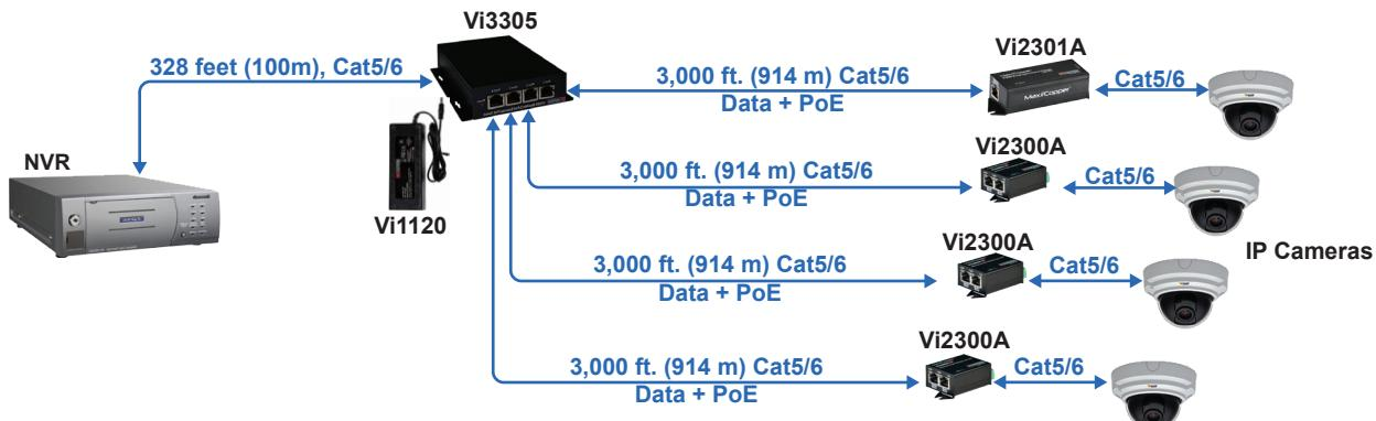
For smaller systems direct connection from Vi3305 to NVR or Computer running VMS can eliminate the need for an extra network switch.
