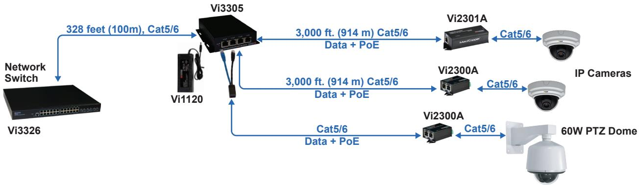
Up to four cameras, including high powered PTZ domes can be remotely powered without the need for local power supplies.
