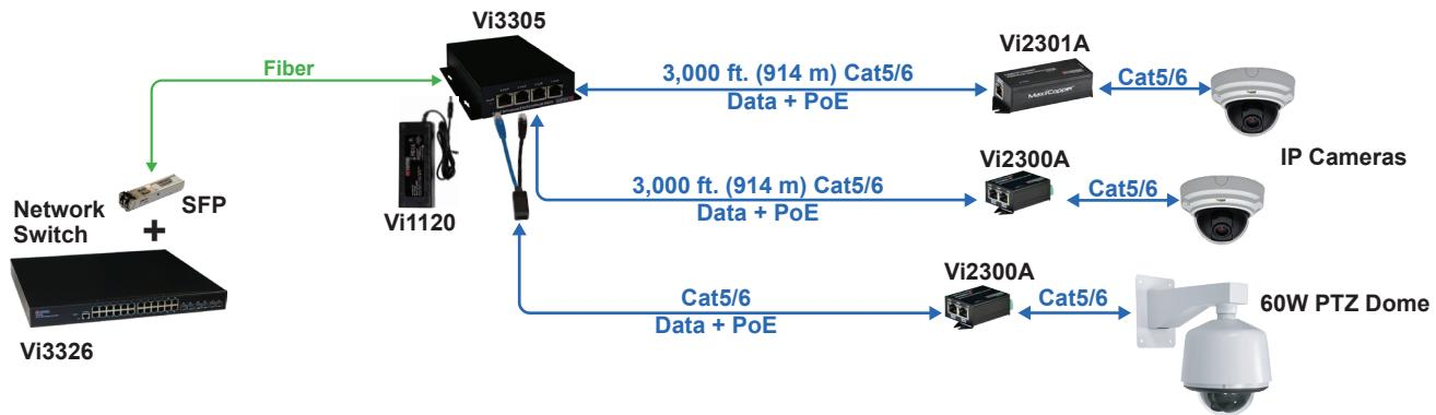
Up/down links can use either the 100Base-T port or Fiber port for distances up to 80Km.
