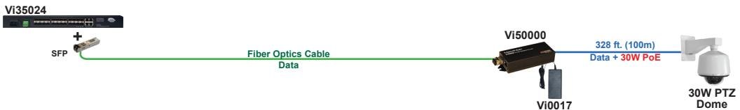
Vigitron Fiber to UTP media converters can be used with Vi35024 to provide 30W of PoE power to cameras or other PoE devices.
