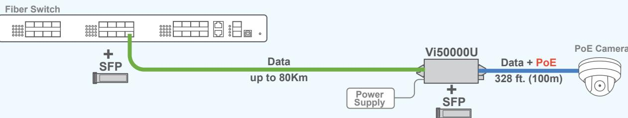
By using the SFPs, the Vi50000U will be compatible with most installed fiber types and can be directly connected to SFP modules installed in network switches.
