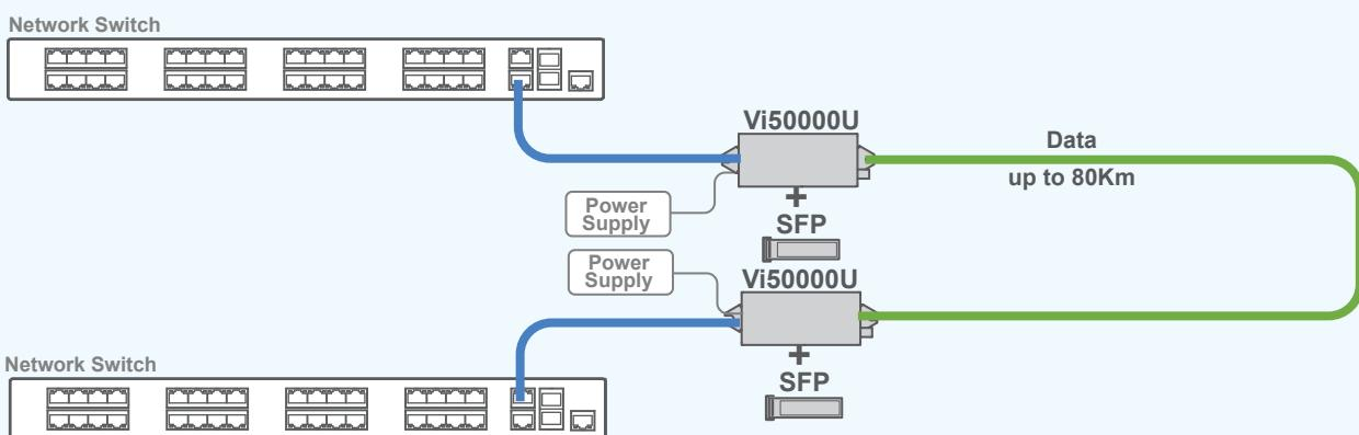
With 1000Mbps (1G) bandwidth, the Vi50000U is the perfect solution for connecting network switches over long distances.
