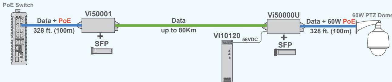
The Vi50000U is used with the Vi50001 for long distance high bandwidth applications. The Vi50000U provides up to 65W PoE power to meet the highest PTZ dome power requirements.
