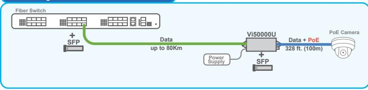
By using the SFPs, the Vi50000U will be compatible with most installed fiber types and can be directly connected to SFP modules installed in network switches.
