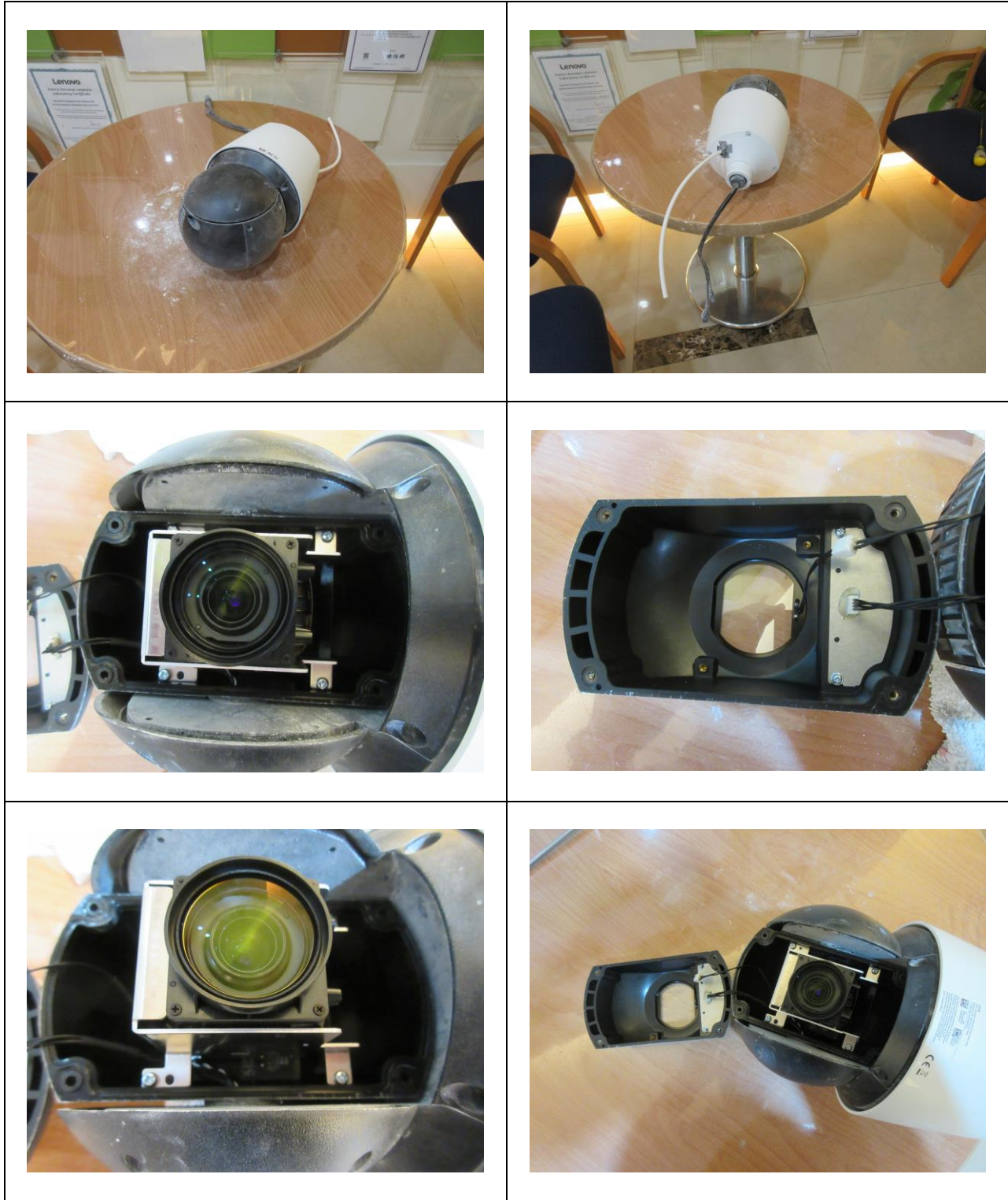
Photo of EUT after dust test
