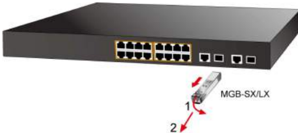
Figure 2-8 How to Pull Out the SFP Transceiver
