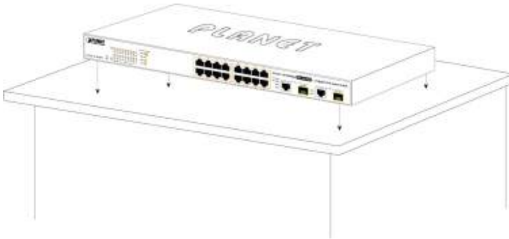
Figure 2-4 Place the PoE Web Smart Switch on the desktop
