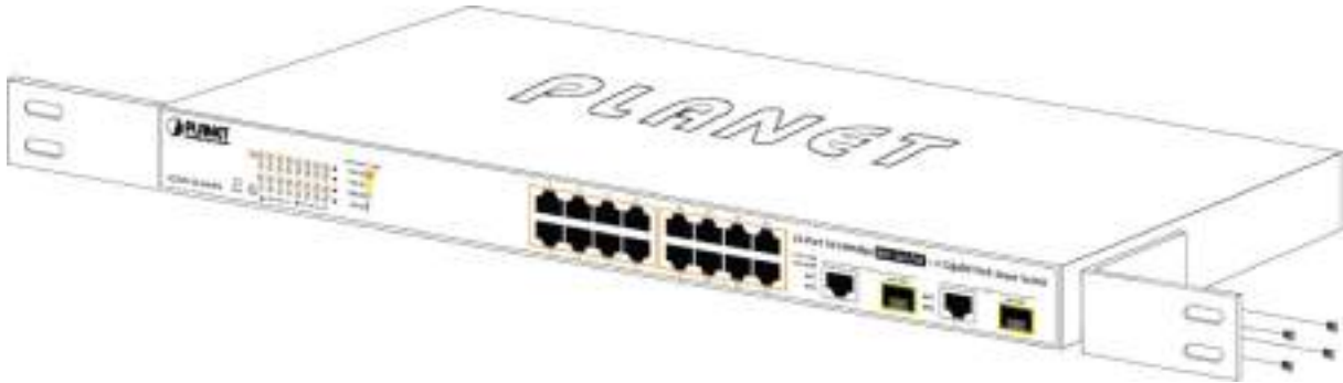
Figure 2-5: Attach Brackets to the PoE Web Smart Switch.
