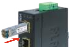
Figure 2-3: Plug-in the SFP Transceiver
