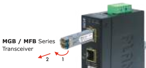
Figure 2-4: Pull Out from the Transceiver
